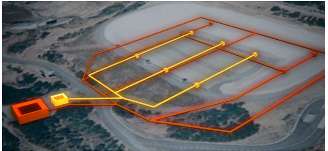
Diagram of the sub-superficial water drainages.
